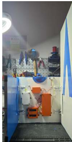
Figure 3.24: Electronics assembled on third module, music module
