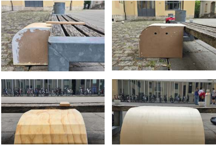
Figure 3.17: (Left) Failed curved module, (Right) Remade module
