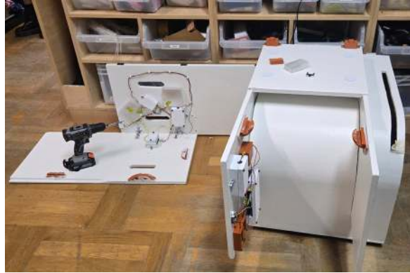
Figure 3.20: Installing electronics on modules
